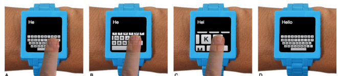
Figure 1: ZoomBoard on a watch-sized device. The keyboard is fully zoomed out by default (A). When users press a key, the keyboard iteratively zooms in (B & C), until the keys are a size that is comfortable and accurate (C). After the desired character is entered, the keyboard resets (D). Users may also swipe to the left to delete, to the right for a space, and up to switch to a symbols keyboard.
