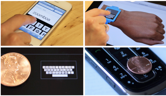
Figure 2: ZoomBoard could be used on a variety of device sizes, for example a smartphone (top left), watch (top right; simulated on a iPad), or coin-sized (bottom left). For size comparison, a typical physical number keypad (bottom right).
