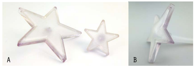
Figure 10. Star buttons fabricated with auxiliary support (A). The big star is inflated in (B) at 0.6 psi (4.1 kPa) relative to atmospheric pressure.
