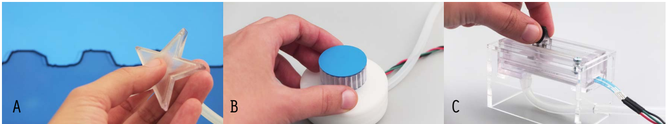
Figure 1. 3D printed pneumatic button (A), knob (B), and slider (C). We print these models with rigid and elastic materials, and in some cases add electronic components to the controls to sense user’s input, such as potentiometers in the case of (B) and (C). Pressure sensing can be used to detect when users deform the elastic parts of the controls, like when they push the star. The graph behind this model shows the sensed pressure signal. We also use pressure to provide variable activation force capabilities.
