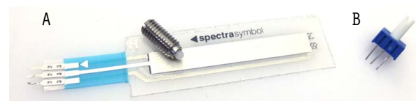
Figure 3. Off-the-shelf potentiometers used in some of our controls: SpectraSymbol's linear sensor and wiper (A), and rotary sensor (B).
