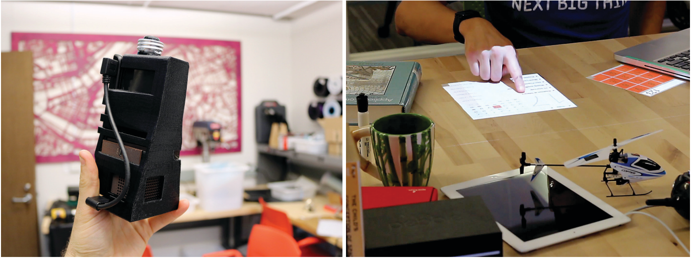
Figure 7. Proof-of-concept “infobulb” (left) able to project multitouch interfaces onto everyday surfaces (right).
