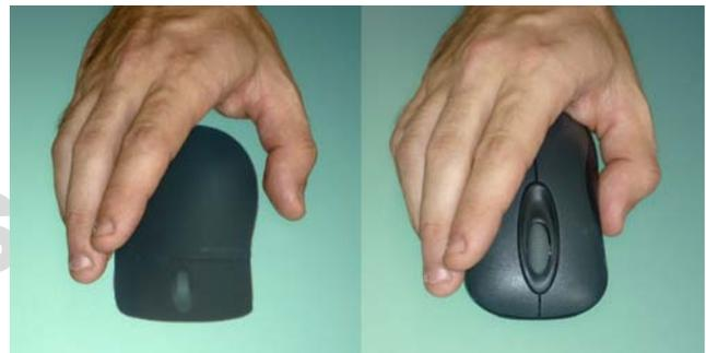
Figure 1. SurfaceMouse (left), Physical Mouse (right).
