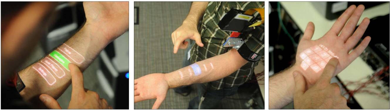
Figure 11: Our sensing armband augmented with a pico-projector; this allows interactive elements to be rendered on the skin.
